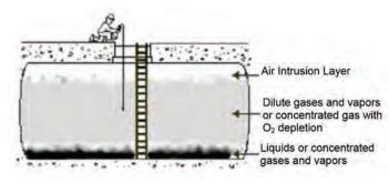
Before entering the confined space, take samples at several levels, and after entering, monitor the space continuously because conditions can change.
